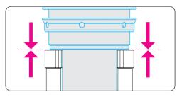
Make sure that the vehicle is supported upon the elephant feet before operating any maintenance.
