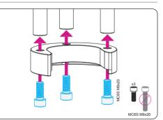
MC6S M8x20 stainless steel bolts to connect the bottom part to the full assembly
