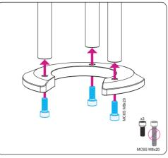
Now locate the bottom foot of the elephant foot and align it with the three leg rods and use three of the included MC6S M8x20 stainless steel bolts to connect the bottom aluminum foot to the assembly.
